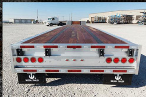
Roadbrute and Premier drop decks are standard with an extruded aluminum rear end with aluminum R.I.G. (Steel R.I.G. is optional on the Roadbrute.)
