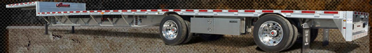
The Premier AD-1080 All Aluminum drop deck – This is what an all aluminum drop deck product should be – A full capacity product able to carry an evenly loaded capacity of 80,000 pounds and a concentrated load of 50,000 pounds in 4 feet of space.
