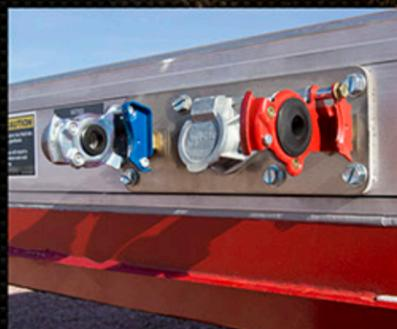
Wilson's redesigned front end has a cleaner, lower profile with gladhand and electrical hookups mounted on a removable access plate
