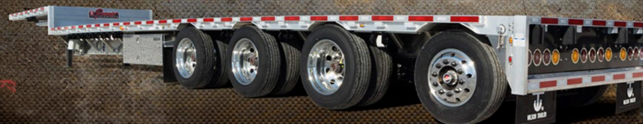
Wilson offers a variety of optional suspensions designed to make the most of gross weight limitations depending on your locale. For extreme hauling Wilson offers a quad axle suspension with steerable rear lift as shown above.
