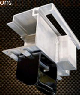
A "Quick Tie" plate receiving rail, located in the outside rail and below floor level, allows wider loads to be secured at multiple locations along the rail and not be susceptible to mud, ice and gunk build-up. The large cutouts in the outside rail easily fit 4" wide winch straps.
