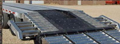
Optional lowered center floor section will allow grain cart undercarriages to clear the transition of the beavertail to the main deck.
