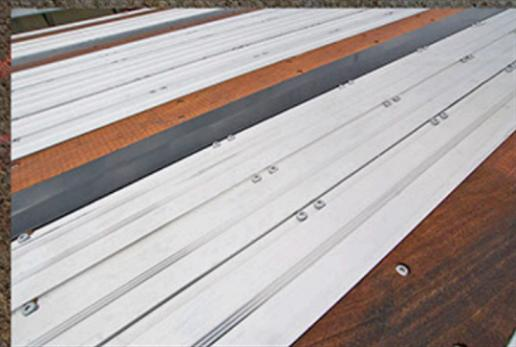
The floors of the Roadbrute and Premier are made of 1-3/8" thick extruded aluminum flooring material with apitong nailer strips, both running the full length of the trailer without any splices. This makes the trailer very stable and successfully reduces side sway.
