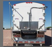
Side Swing Door with Hydraulic Slide Gate and Cathedral Header
