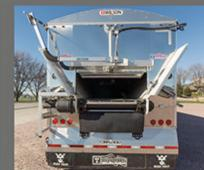
Top Hinge with Hydraulic Slide Gate and Optional Stainless Rear
